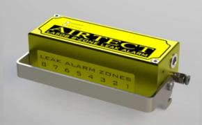
LA508-M-H—N 8-ZONE MODULAR LEAK ALARM MANIFOLD (requires connection to an LA500, LA502 or LM2050 IMM Nozzle Leak Detector Module via a PCC-X Cable. Requires an LA508-B-X base). Kit Includes:
